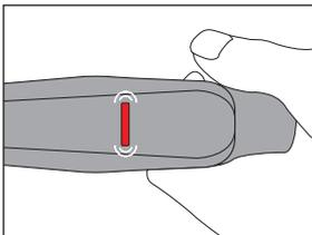
Flashing red light: The rechargeable battery needs to be charged.
