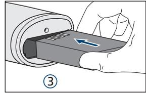
Install the battery and close the battery compartment lid.
